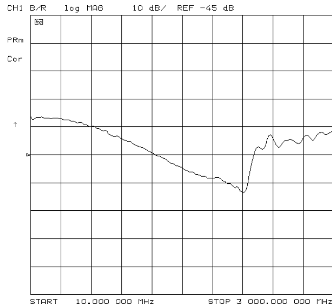
Figure 2-36 Example Mixer LO to RF Isolation Measurement
